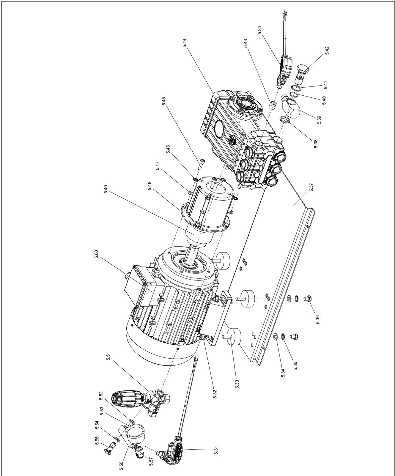
Fig. 10 - 6 Drive unit motor and pump, exploded view
