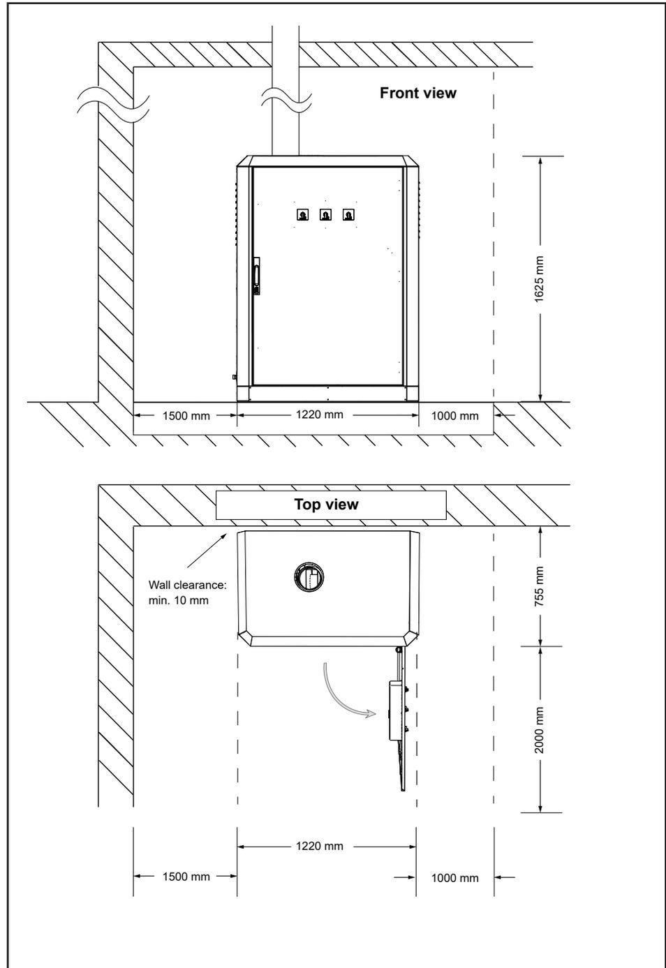
Fig. 4 - 1 Required dimensions for system operating location
