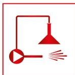
**High-Pressure Chemical with Dosing-Valve** Any cleaning-detergents can be applied during high-pressure stage by opening the Dosing-Valve. The High-Pressure Pump will absorb detergents together with water and pressurize it.
